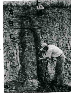
A loessial soil profile with A, B, and C horizons being sampled for tests with soil-cement. Biological activity ordinarily centers in the A.
